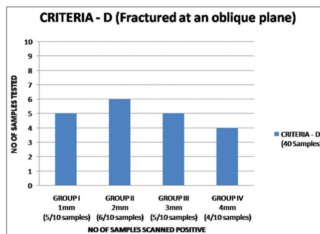
Figure 11: Graph demonstrating result when samples containing QR codes were fractured (Criterion D)
