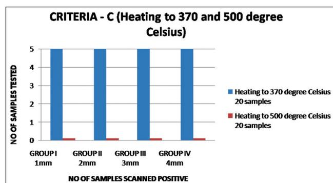
Figure 10: Graph demonstrating result when QR codes were heated drastically (Criterion C)
