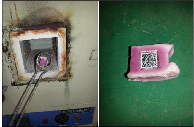
Figure 5: Sample heated to 370°C, QR code not destroyed
