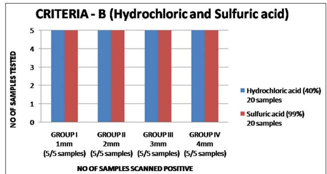
Figure 9: Graph demonstrating result when QR codes were exposed to inorganic acids (Criterion B)
